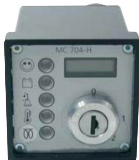
Temporary errors will be ignored and stay accumulated for 10 seconds. If they exceed 3 seconds in total in this time the engine will be shut down automatically and the alarm will be activated.
